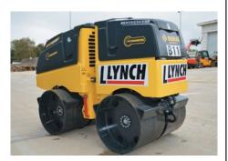
Additionally the operator knows when compaction is finished as the 'Bomag Economizer' automatically determines compaction progress. Expensive reworking is no longer necessary and over compaction and unnecessary passes are also avoided, resulting in time savings of up to 25%.
