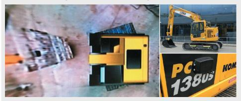
In response to a direct request from Balfour Beatty to investigate safer options when slewing, Lynch is the very first plant hire company to install Brigade's Backeye®360 camera and Radar OSD (On-Screen Display) vehicle safety systems to one of its Komatsu excavators. This particular one is now on route to be used in Balfour Beatty's training area on the M4!
