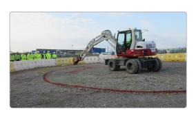
This shows the working radius of the excavator.
